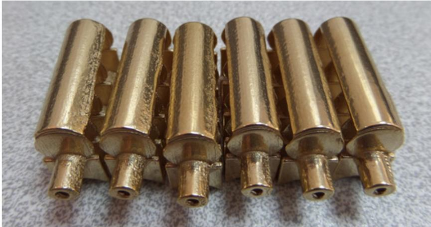
*Samples polished with ceramic media with increasing polishing time from left to right*
