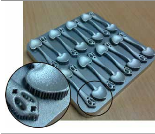
Figure 22 Building silver spoons arranged face up requires a huge number of supports and subsequent finishing effort. Image is courtesy of ES Technology.
